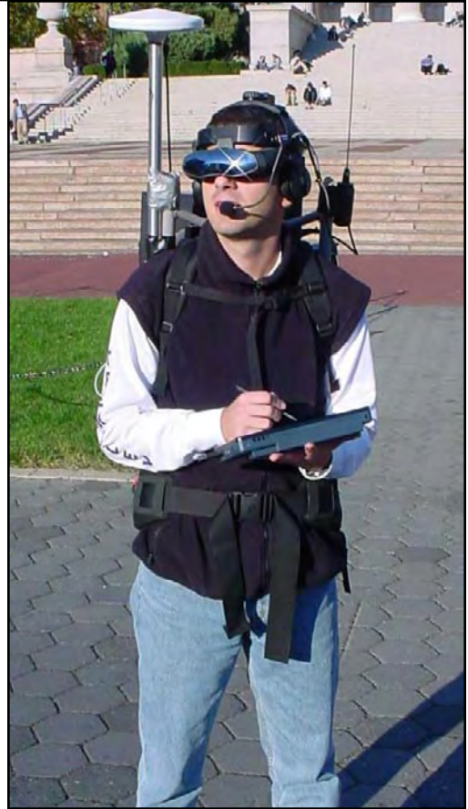
Backpack of the future: Experimental equipment for mobile augmented reality systems. A much more compact system has since been created.
